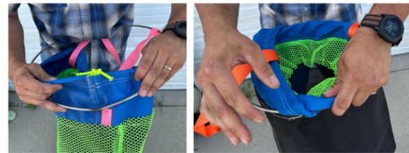
Roll the head of the bag over the top of the hoop so that the bag is inside the hoop and thick shock cord is outside the hoop
