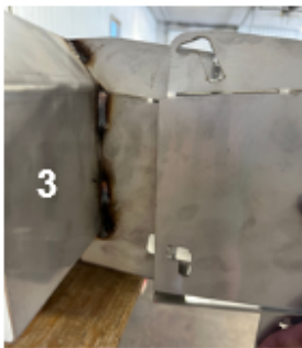
3. Slide bottom thumbs into finger lock slot
